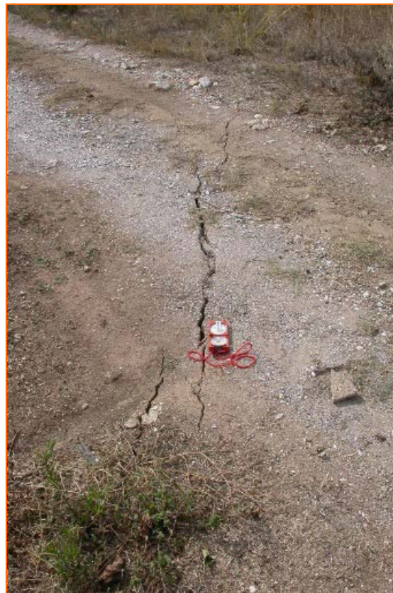
Coseismic surface ruptures and offsets south of Agios Nikolaos village (left) and in the coastal zone of Agios Nikolaos (middle).
